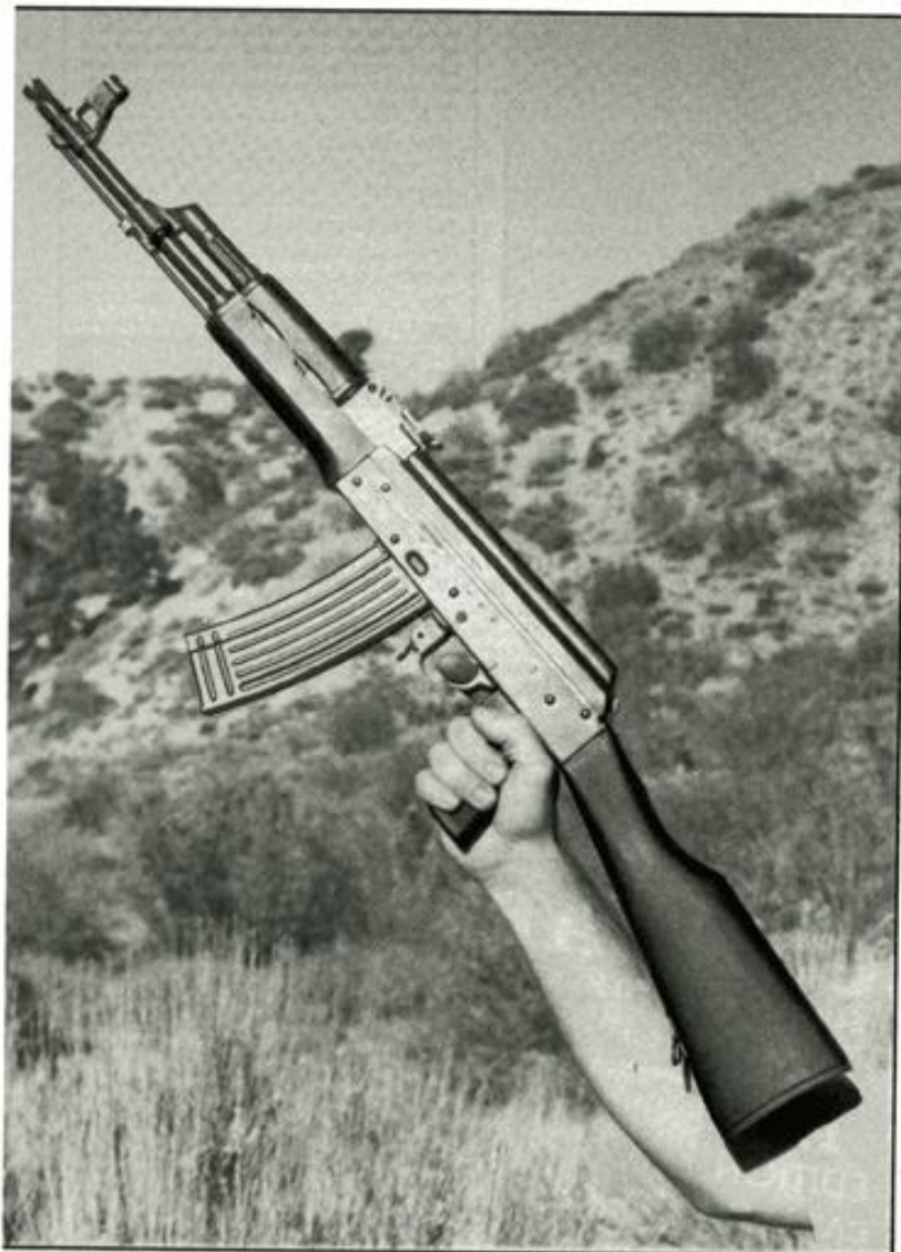
The Type 84S .223 AK-47 rifle has a butt stock that is 1½-inches longer than the standard AK butt stock.
