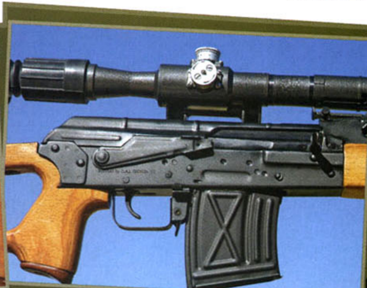
Left: Mechanically, the Romanian PSL is based on the AKM platform rather than on the original Russian Dragunov design. The stamped PSL receiver is reinforced at the rear with two steel plates just ahead of the buttstock.
